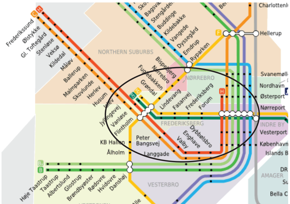
Figure 4-22: Schematics of the public transport network where S-train and metro overlap at Vanløse st, Flintholm st. and Nørreport st. but not in between.
