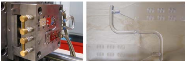
Figure 2. Two-cavity flexible mould with both coated and non-coated micro Fresnel nickel tool inserts mounted (left); two-parts moulded parts: the six pairs of micro Fresnel lenses are visible on the surface of both components (material = polycarbonate).
