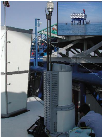
Lidar wind data and model from Horn's Reef offshore
