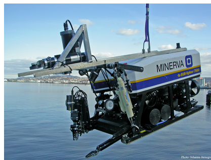
Fig. 1. ROV Minerva 1 , a SUB-fighter 7500 ROV from Sperre A/S. Photo: Johanna Järnegren
