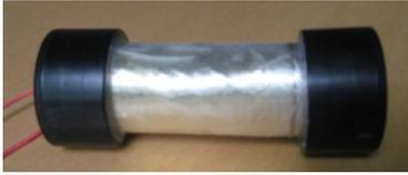
**Figure 2.** PolyPower DE tubular actuator
