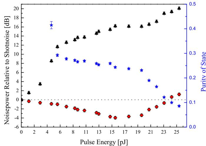
Fig. 3. Measured noise power versus the optical pulse energy. Red squares and black triangles show squeezing and anti-squeezing, respectively (left scale). We observed a maximal squeezing of  $-3.9 \pm 0.3$  dB with an anti-squeezing of  $16.2 \pm 0.3$  dB. The blue stars show the purity of the squeezed state (right scale). All data is measured at a frequency of 17 MHz. The squeezing is only corrected for electronic detector noise which is 13 dB below the shot noise.
