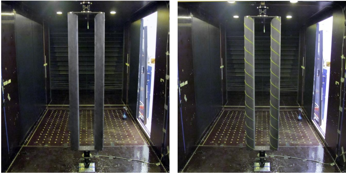
Figure 1: Wind tunnel test setup of twin cylinders without (left) and with (right) double helical fillets for wind angle-of-attack \alpha = 0^\circ .
