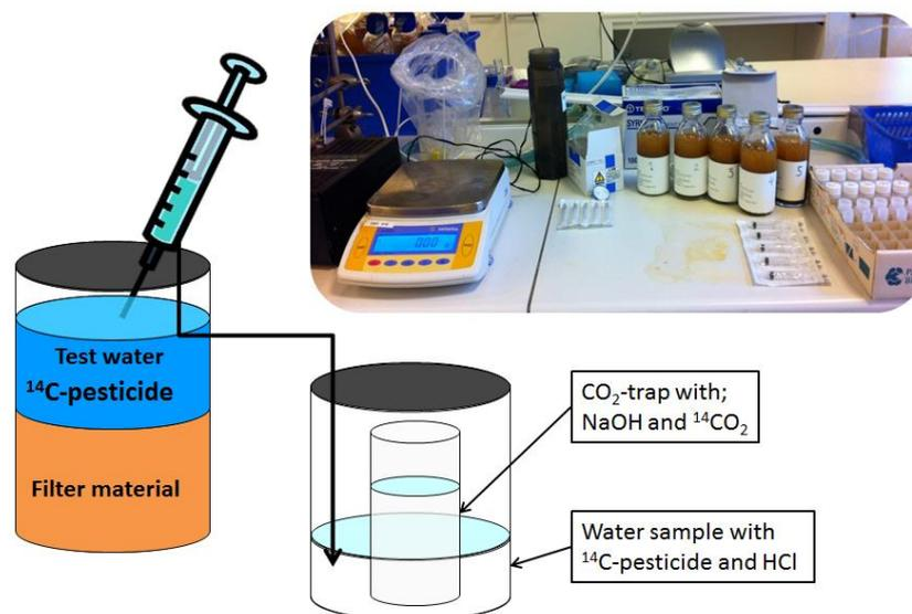
**Figure 2** Microcosms consisting of filter sand, water and  $^{14}\text{C}$ -pesticide. Water samples were collected, filtered and transferred to 20mL plastic vials. HCl was added to water samples to strip off  $^{14}\text{CO}_2$  from mineralisation of  $^{14}\text{C}$ -pesticide and  $^{14}\text{CO}_2$  was caught by a base trap.
