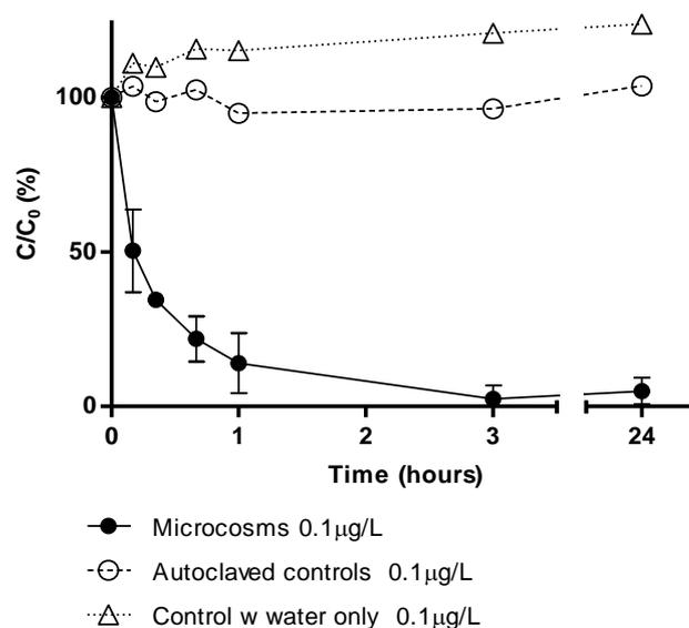
**Figure 3** Removal of bentazone in microcosms consisting of 100 g filter sand and 100 ml water from Sjælsø waterworks Plant II. The mean concentrations and standard deviation are given as percentage of the initial concentration. Microcosms with an initial concentration of 0.1 µg/L (triplicate) are depicted along with two corresponding controls (initial concentration 0.1 µg/L), one with autoclaved filter sand and one with water only.
