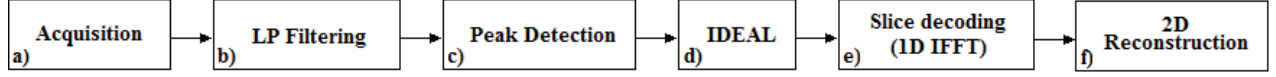
Fig. 2: Diagram of the 3D CSI data processing. a) Acquisition stage. b) Low-Pass filter to improve SNR of acquired data. c) Search for the resonance frequencies. Resonance frequency of the peaks in the spectrum can be achieved using matching pursuit. d) IDEAL implementation using a pseudo-inverse matrix. e) 1D IFFT along slice direction. f) 2D reconstruction of slices separately.
