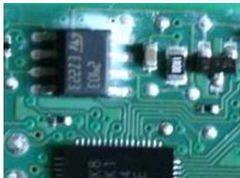
Figure 3 Field failure returned PCBA showing white residues near integrated circuit chip component.
