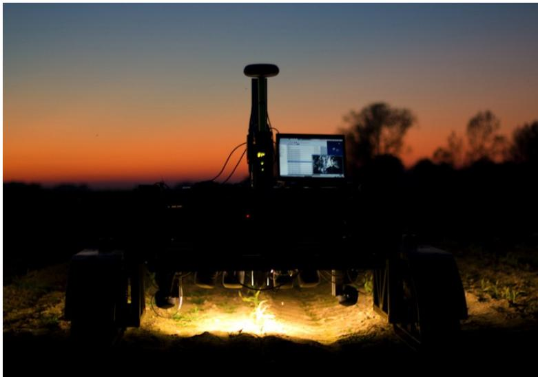
Fig. 8. Armadillo collecting images of weed in a maize field at dusk
