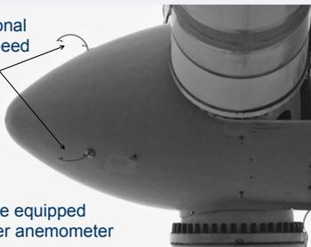
A wind turbine equipped with a Spinner anemometer
