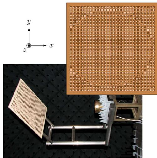
Fig. 5. Reflectarray designed with a pencil beam directed toward  $\theta = -30^\circ$  and  $\phi = 0^\circ$  in the shown coordinate system and measured at the DTU-ESA Spherical Near-Field Antenna Test Facility.
