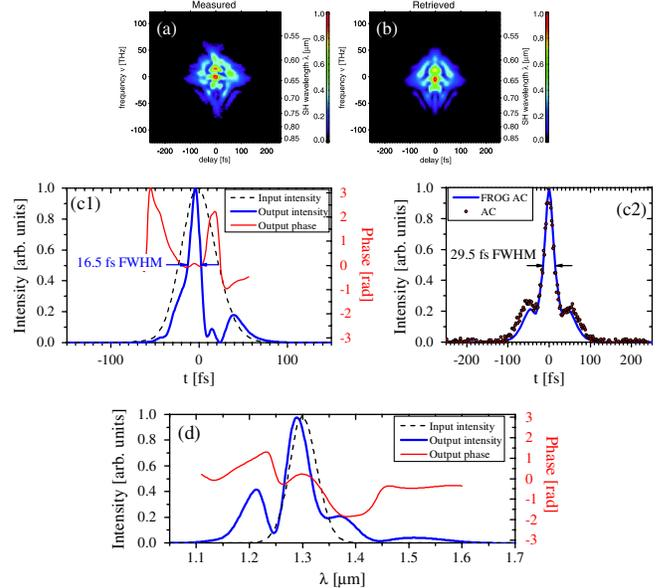
FIG. 3 (color online). FROG measurements at  $I_{\text{in}} = 1.0 \text{ TW}/\text{cm}^2$ : (a),(b) FROG traces (amplitude) of the output pulse. (c1) The temporal and (d) spectral amplitudes and phases retrieved by the FROG algorithm. (c2) The calculated FROG intensity AC and the experimentally measured AC.
