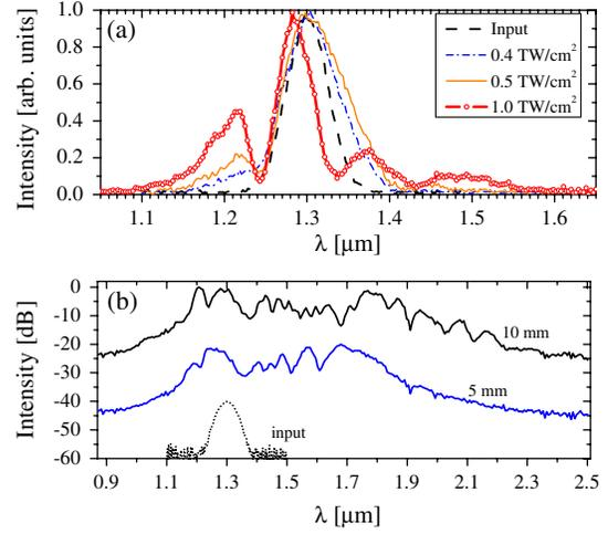
FIG. 2 (color online). (a) Spectra after a 1 mm LN crystal for various input intensities. (b) Spectra after 5 and 10 mm propagation using  $I_{\text{in}} = 1.0 \text{ TW}/\text{cm}^2$  (averaged over 1100 shots). The spectra in (b) are offset 20 dB from each other for clarity.
