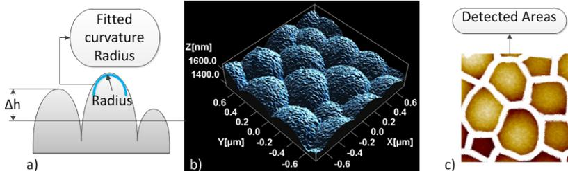
Figure 2: a) Measurement technique to estimate height variation and radius of the fitted features curvature; b) example of  $1,5 \times 1,5 \mu\text{m}^2$  nickel scanned surface; c) texture cells detected on the nickel substrates used to calculate the average area.
