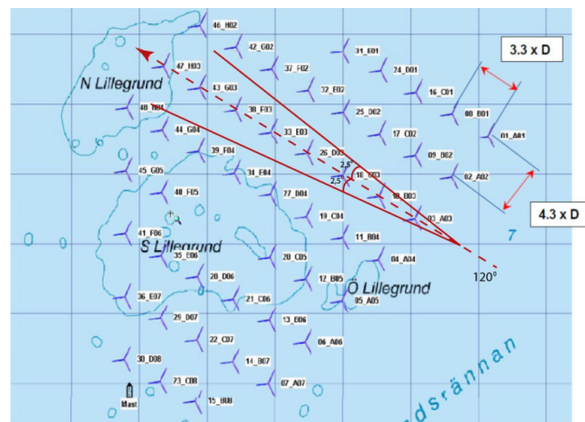
Fig. 1 Location of the 48 wind turbines in Lillgrund, inflow sector 120 \pm 2.5 degrees. [10]
