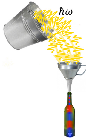
Figure 1. An artistic view of the problem of coupling light from a wide microscopic fiber to a nanoscopic waveguide. Employment of a coupler, which is represented by a funnel on the figure, minimizes the losses and simplifies optical alignment.
