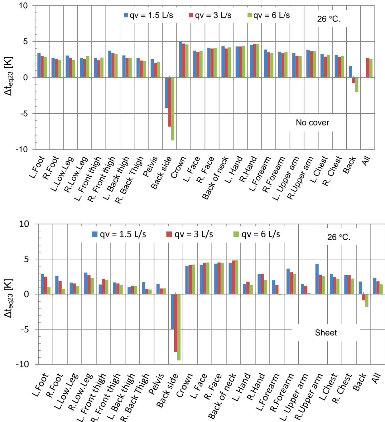
Figure 4. Change in the equivalent temperature,  $\Delta t_{eq2}$ , at room air temperature of 26 °C compared to at room air temperature of 23 °C. VM in operation. Results when the body is covered with sheet and not covered are shown.
