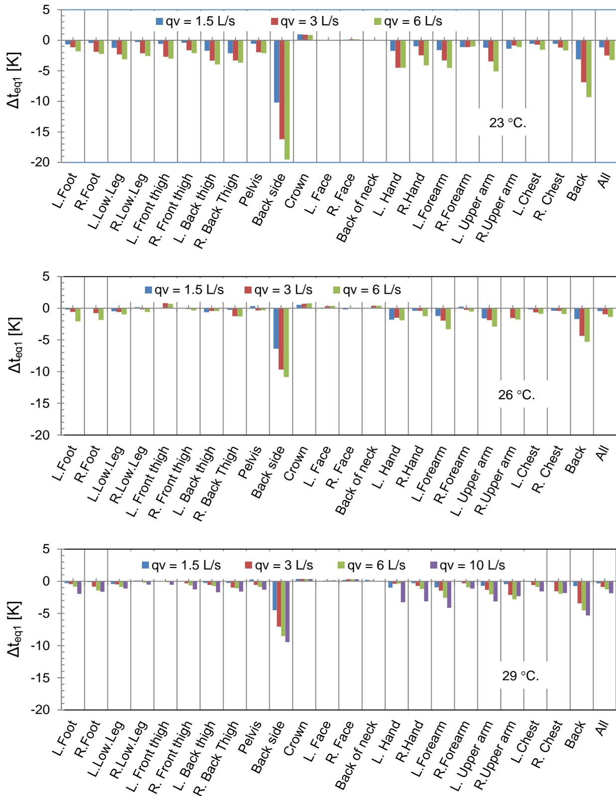
Figure 2. Change in the equivalent temperature,  $\Delta t_{eq1}$ , for manikin's segments and whole body at different flow rates and room air temperature with VM in operation. Manikin covered with sheet.
