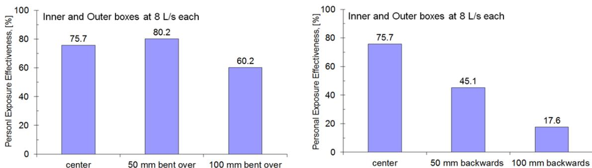
a) b) Figure 3. PEE as a function of the positioning of the thermal breathing manikin a) when moving backwards from the table and b) when bending over the table when the width of both jets are at 0.06 m and both supply at 8 L/s.
