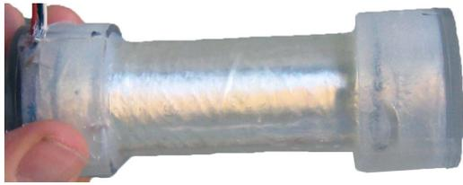
Fig. 1. A prototype of linear DEAP actuator.
