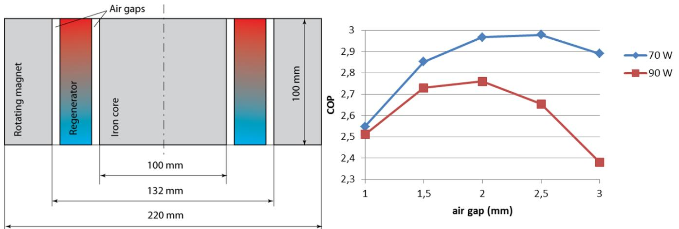
Fig. 2. Regenerator between iron core and rotating magnet. Calculated COP as a function of air gap taking radial heat losses into account for 70 W and 90 W cooling power.
