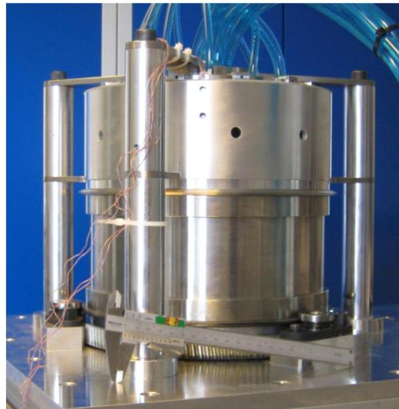
Fig. 1. MAGGIE. Rotating cylinder containing magnet, regenerator and flow handling system.
