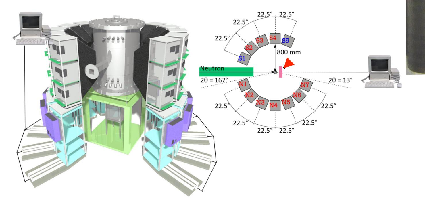
Setup used at BL18. Data were acquired simultaneously by near- (indicated by red arrow) and far-field detectors.
