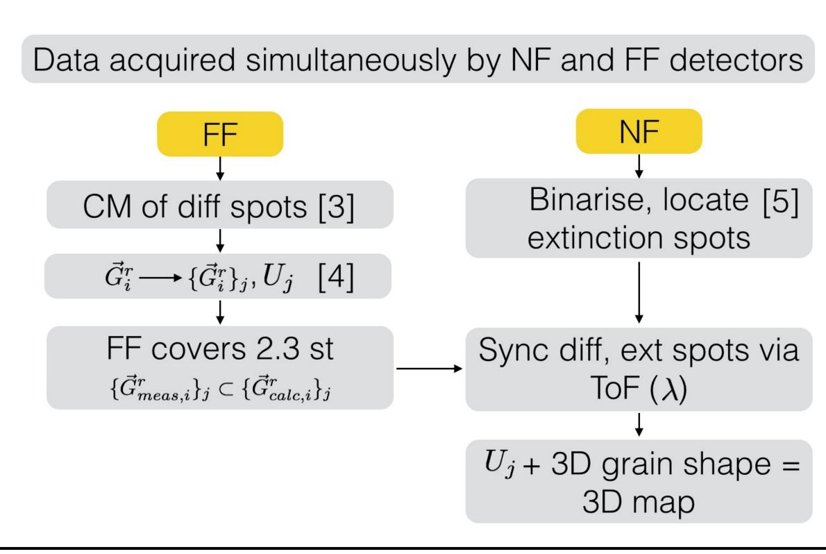
3DND is a nondestructive technique to investigate, in a reasonable time frame, the 3D structure of mm- to cm-sized polycrystalline samples. It completes existing X-ray techniques, enabling to use complex sample environments. Combined with a time-of-flight beam, 3DND can be used to study samples composed by a large number of grains. Once the reconstruction algorithm is fully implemented, we will apply 3DND to study shape memory alloys.
