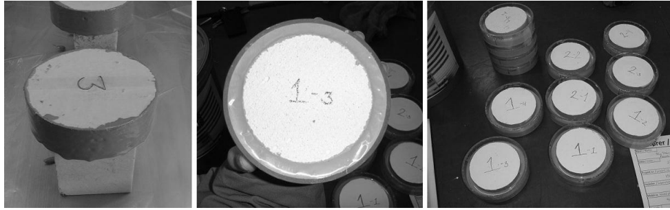
FIG 2 Specimens to the cup tests. Left: Specimen, which has just been painted with epoxy on the vertical perimeter surface sides. Middle: Specimen placed in a plexi glass ring with epoxy between the specimen and the plexi glass ring. Right: Specimens ready for the cup test.
