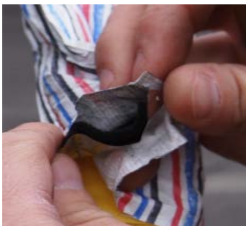
Figure 1: (Left) NAPL-FLUTE liner (a color striped membrane) in combination with the activated carbon strip (FACT). (Right) Simulation results showing two FACTs in a borehole after an exposure time of 42 h in an aquifer with an initially uniform dissolved PCE concentration. The blue arrows mark the groundwater flow velocity.
