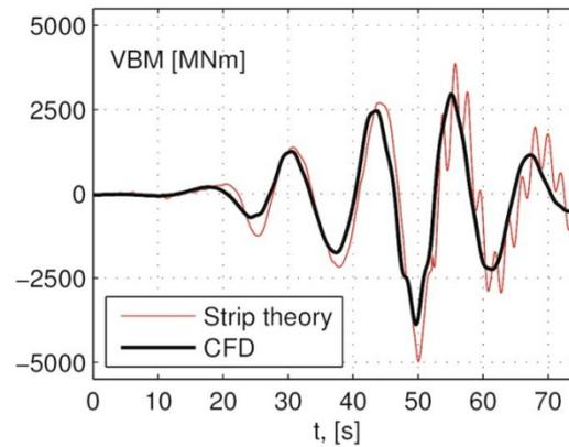
Fig. 2 The vertical wave bending moment conditioned on a vertical bending moment of 5,000  $MNm$  at 50  $\text{sec}$ . In sagging condition. The conditional wave used in CFD is the one obtained using strip theory.
