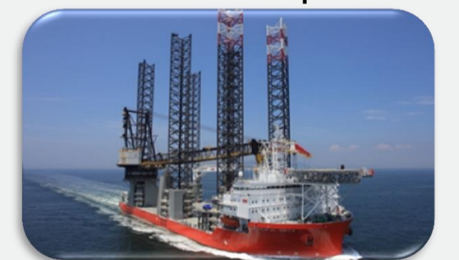
Figur 2: Innovation bio. of Pacific Orca, Swire Blue Ocean Pacific Orca is an offshore installation vessel. Six 105 m legs makes it safe to operate in wind up to 20 m/s.
