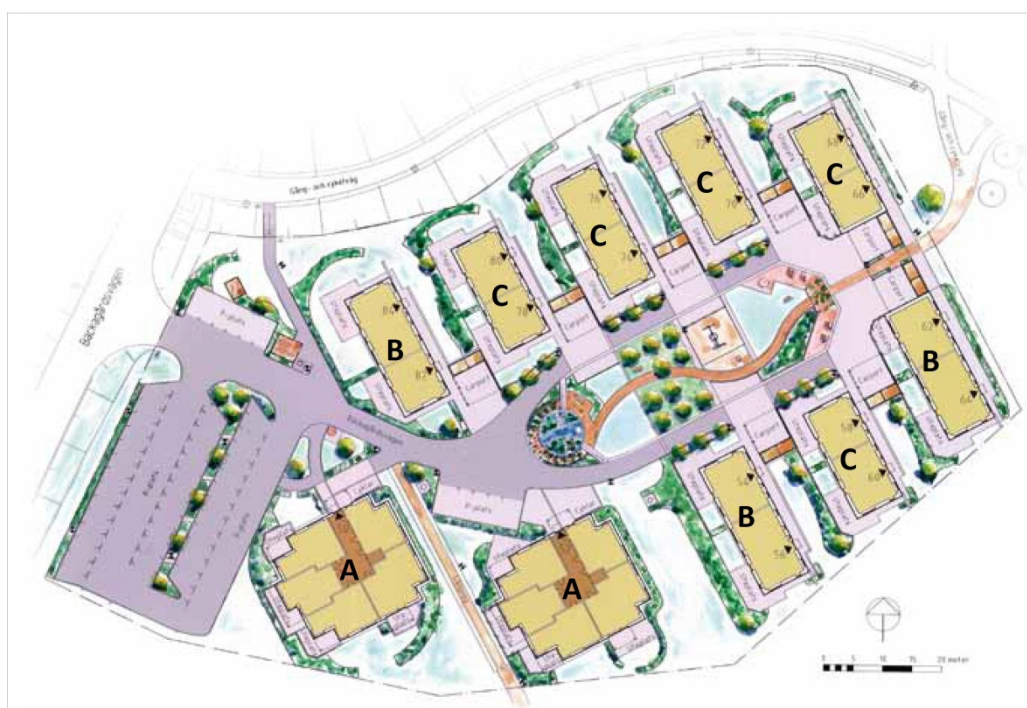
Figure 2. Principal site plan of the Söndrums Kyrkby multi-family and pair passive house ground site. Building types are: (A) Multi-family houses, (B) Pair-houses with a two-room and a four-room apartment, and (C) Pair-houses with two three-room apartments. Source: [3].
