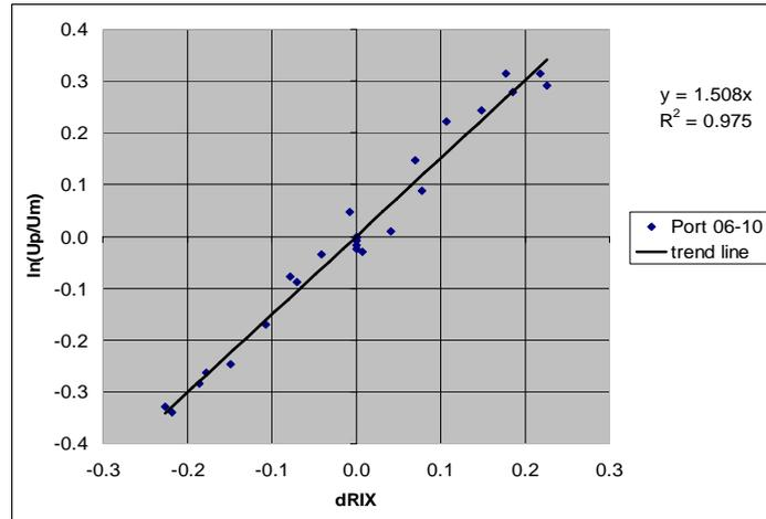
Figure 5. WASP wind speed prediction error as a function of the difference in ruggedness indices,  $\Delta RIX$ , between the predicted site and the predictor site in a log-linear plot. Note, that the  $\Delta RIX$  values are given as fractions here.
