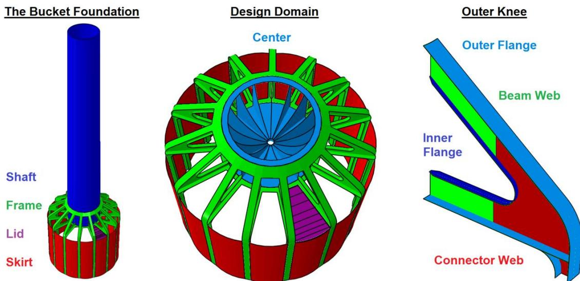
Figure 1 – a) The Bucket Foundation b) Design Domain c) The Outer Knee
