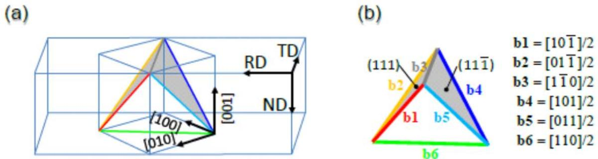
Fig. 1. a) Slip system geometry in plane strain compression and b) colour coding of Burgers vectors for the 45° ND rotated Cube orientation. The two active slip planes (111) and (11 $\bar{1}$ ) are coloured grey. From (C. Hong, Huang, and Winther 2013).
