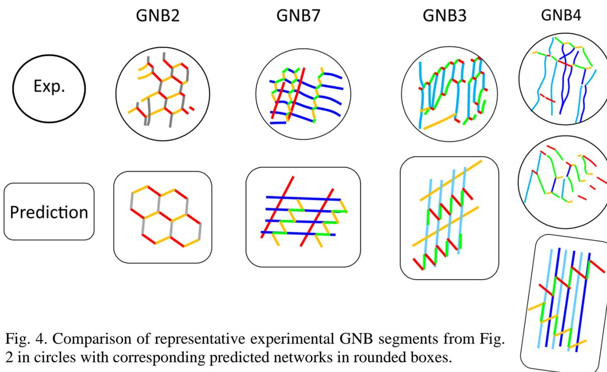
Fig. 4. Comparison of representative experimental GNB segments from Fig. 2 in circles with corresponding predicted networks in rounded boxes.
