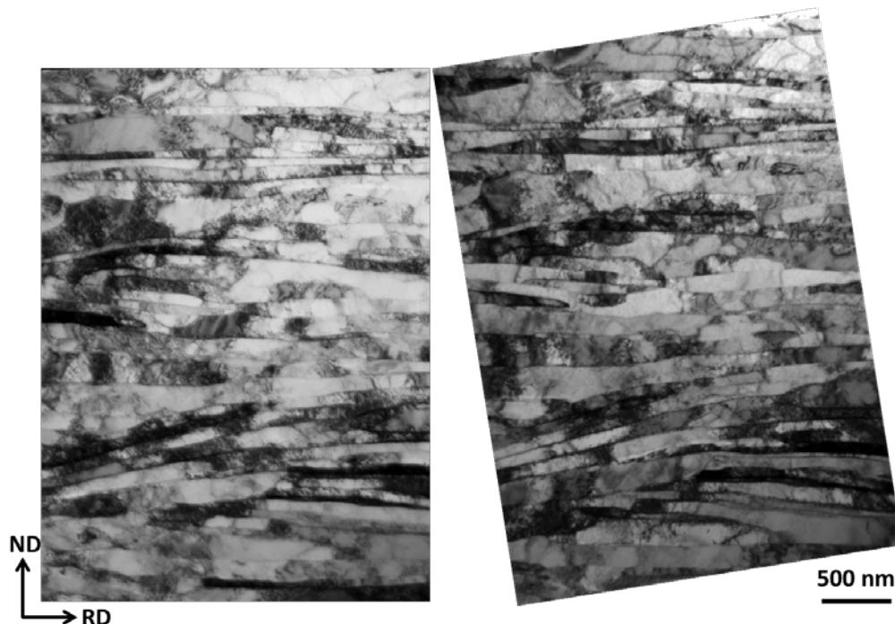
Fig. 1. TEM images showing the microstructure in one region of the ARB-processed nickel sample investigated after different periods of storage: (a) 4 months and (b) 4.5 years after deformation.
