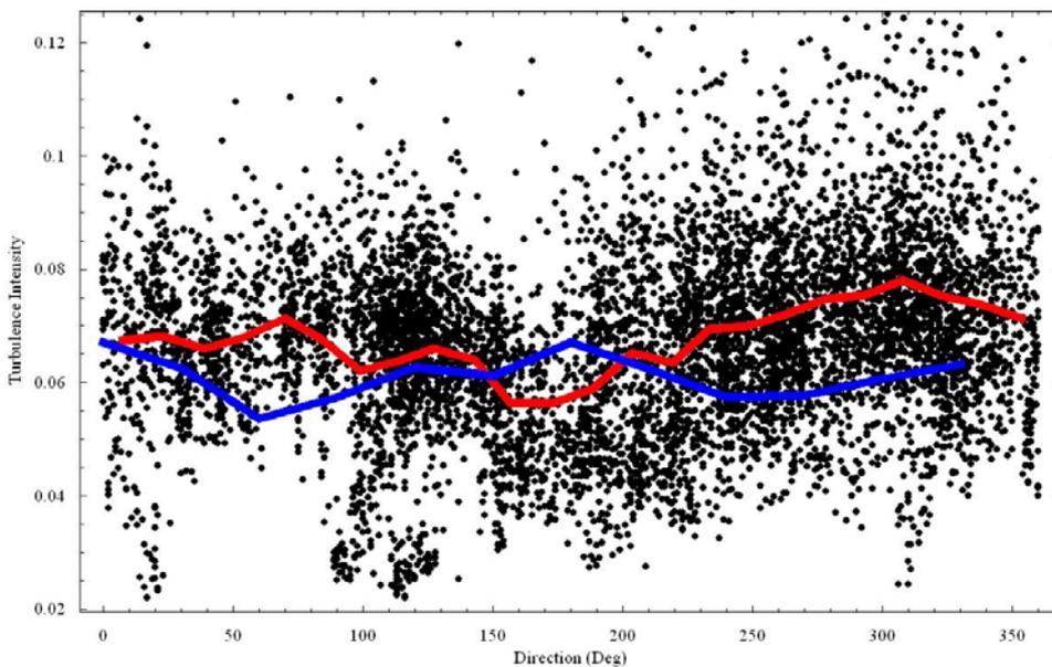
Figure 3. Shows the measured turbulence intensity at 69 meters at Horns Rev versus direction (before the wind farm installation). The measurements are show for wind speeds from 10 to 15  $ms^{-1}$ ; the red curve is the average and the blue is the corresponding WASP Engineering model.
