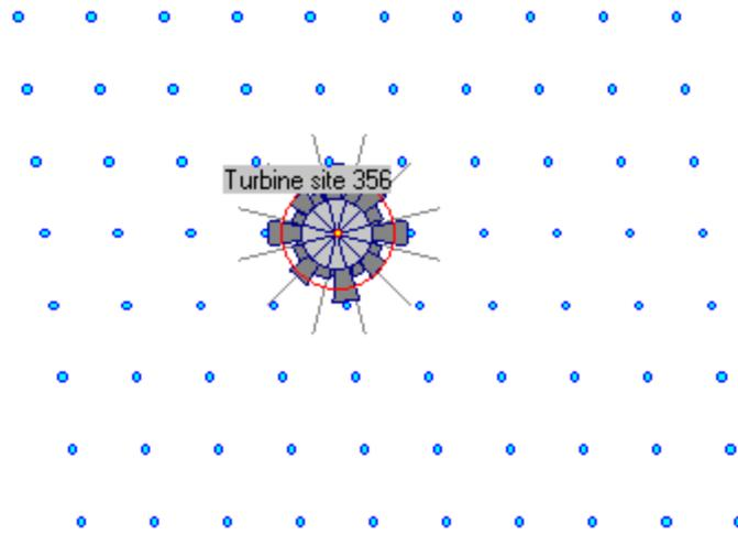
Figure 4. Turbulence intensity at Horns Rev site 356 as a function of wind direction for a wind speed of  $5 \text{ ms}^{-1}$ . Dark grey indicates wake-induced turbulence and light grey indicates free-stream ambient turbulence calculated by WASP Engineering. The red circle indicates the effective turbulence intensity for a Wöhler-curve exponent of  $m=4$ .
