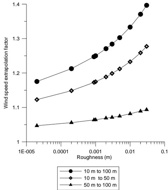
Figure 1. Wind speed profile extrapolation factors for different heights and different roughness lengths assuming a logarithmic profile applies.
