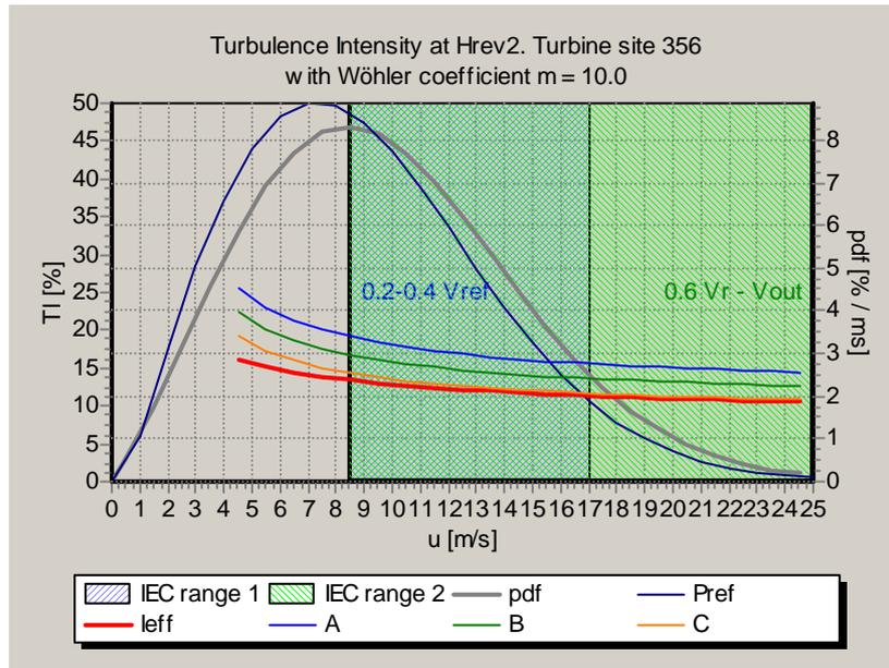
Figure 6. Effective turbulence intensity at Horns Rev turbine site 356, with Wöhler coefficient  $m=4$ . The curves labelled A to C are effective turbulence intensities of the IEC normal turbulence model for the standard wind turbine classes.
