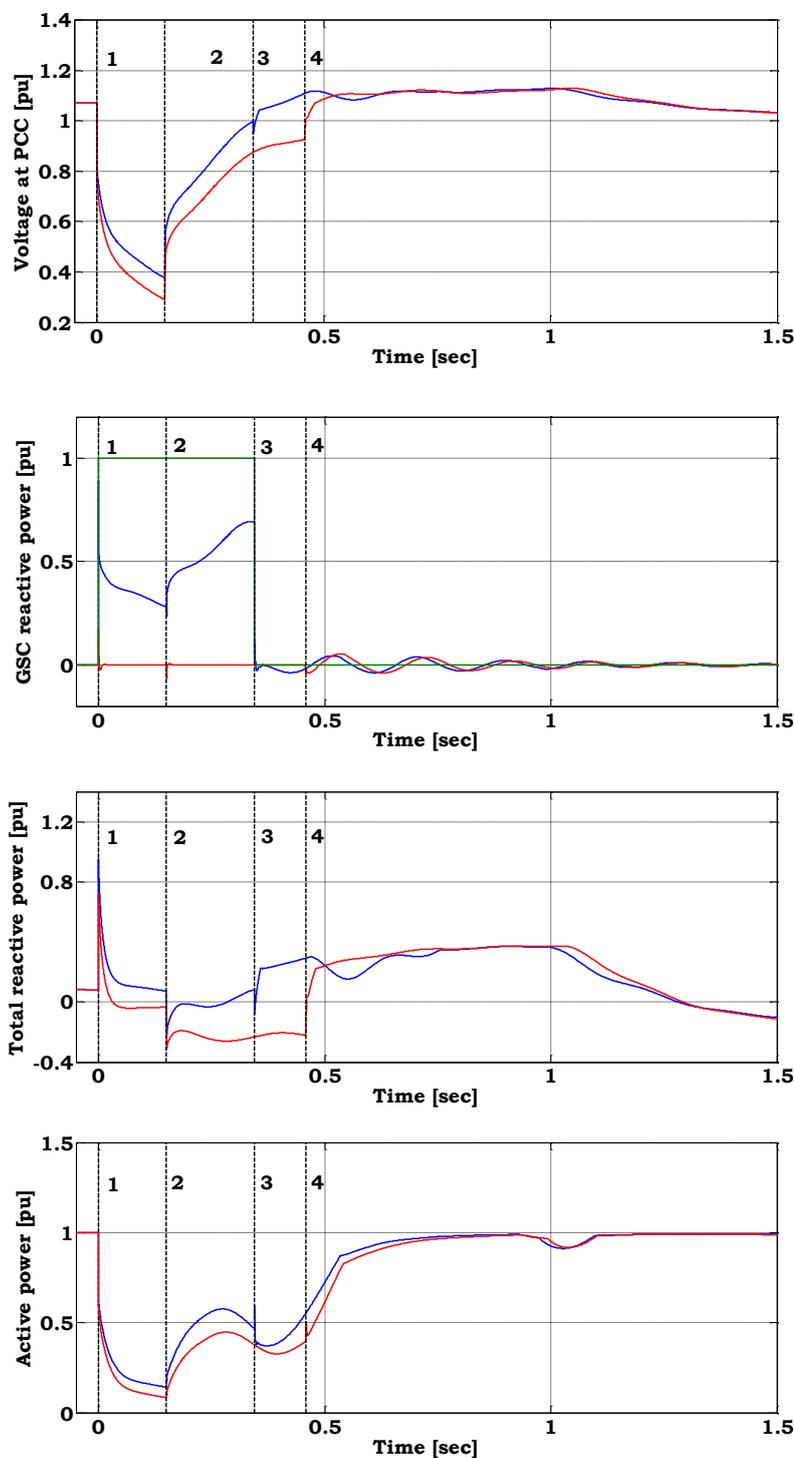
After fault clearing, when the voltage at the converter terminals re-establishes, the GSC is able to provide even more reactive power to the grid. Due to the reactive power demand of the generator, when the fault is cleared, the voltage does not completely recover immediately. The generator operates
