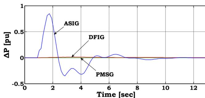
As described in [15,16], the response of a DFIG wind turbine is very different than of ASIG wind turbines. Its inertia is mostly based on the applied control scheme acting on the converter connecting the rotor to the grid. Supplementary control attributes have been proposed in the literature in order to achieve active frequency control by variable speed wind turbines [17,18]. In this article two different frequency control methods are presented for the DFIG wind turbine configuration:
