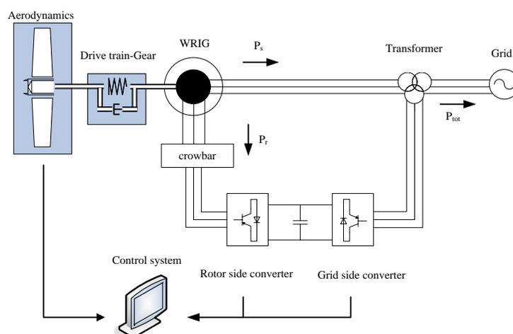
The DFIG system is essentially a wound rotor induction generator with slip rings, with the stator directly connected to the grid and with the rotor interfaced through a back-to-back partial-scale power converter [8]. The converter consists of two conventional voltage source converters (rotor-side converter RSC and grid-side converter GSC) and a DC-bus.
