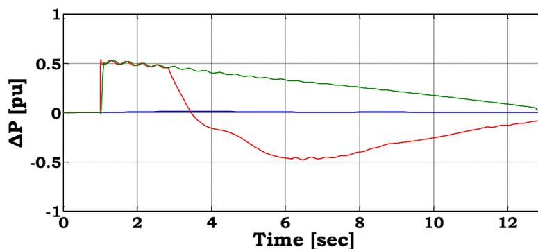
Notice that when no auxiliary frequency control is applied, the frequency drops below 48.5 Hz, leading to load shedding which prevents further frequency drop. In the other two cases, where the frequency control is activated in the DFIG wind farms, the load shedding is totally avoided. The optimum frequency drop in terms of minimum frequency is achieved through droop control.
