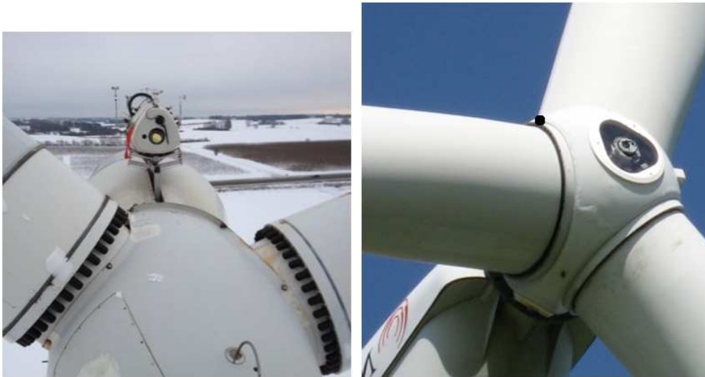
Figure 63: Continuous wave dual mode ZephIR 300 lidars mounted on a nacelle roof (left) and within a wind turbine spinner (right).
