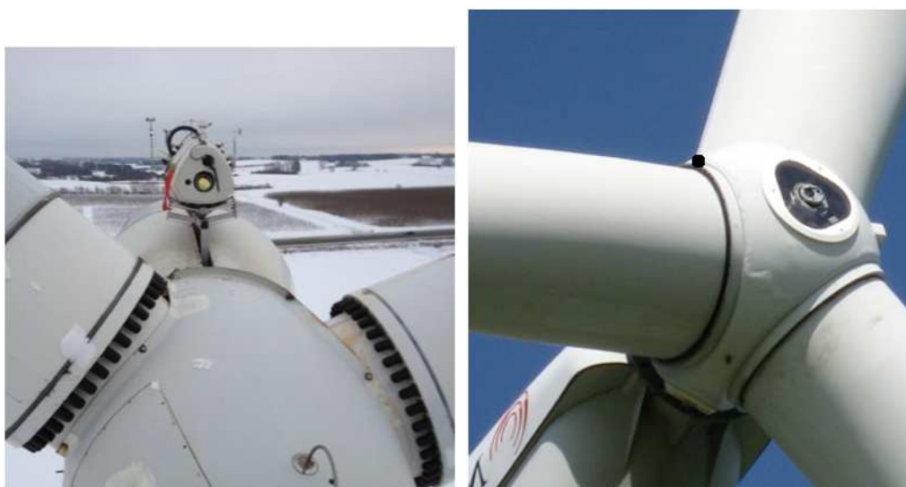
Figure 63: Continuous wave dual mode ZephIR 300 lidars mounted on a nacelle roof (left) and within a wind turbine spinner (right).
