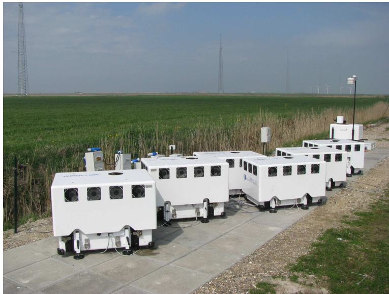
Figure 7: Pulsed wind lidars (six WLS7 WindCubes) and one Galion (far back) during testing at Høvsøre, Risø DTU
