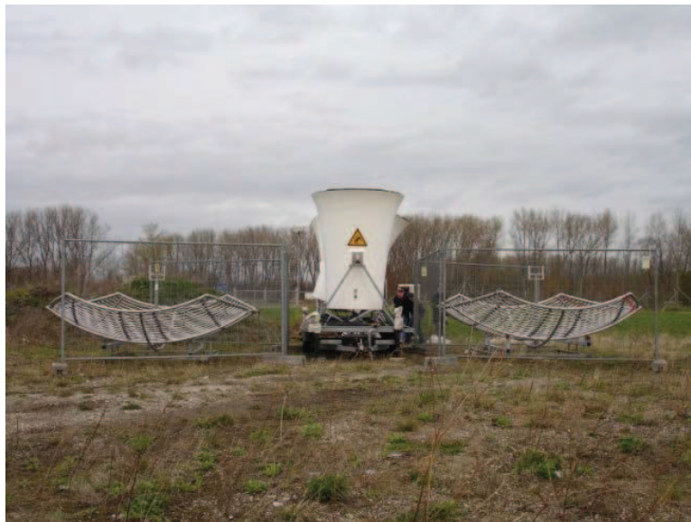
Figure 87: Sodar-RASS. The acoustic antenna is in the middle, the electro-magnetic antennas to the left and right.
