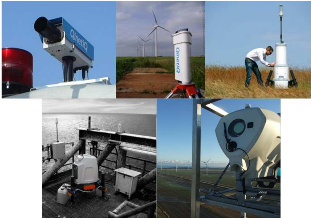
Figure 55: Stages of evolution of the ZephIR lidar. The upper left-hand picture (a) shows the lidar head mounted on the nacelle of a Nordex N-90 wind turbine (March 2003). The top central picture (b) shows a prototype ground-based wind profiler at the Risø wind energy test site at Høvsøre, Denmark. The top right picture (c) shows an early ZephIR production model deployed in the field. The lower pictures show a more recent dual mode ZephIR DM300 deployed on an offshore platform (d) and on a turbine nacelle (e).
