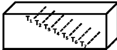
Figure 1 Geometrical setup of the experiments in the blast cooler
