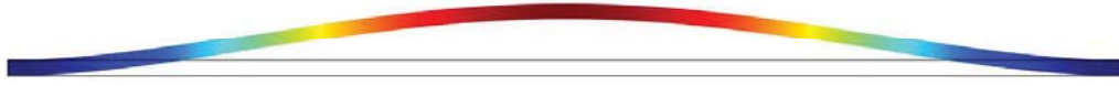
Figure 2. Initial design of a clamped-clamped beam and its linear vibration mode. The color in online version indicates the vibration amplitude.
