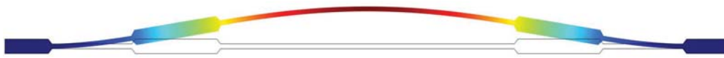
Figure 3. Optimized design for maximizing the cubic nonlinearity of a clamped-clamped beam and its linear vibration mode. The color in online version indicates the vibration amplitude.
