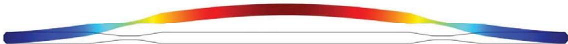
Figure 6.3 Optimized design for minimizing the cubic nonlinearity of a clamped-clamped beam and its linear vibration mode. The color represents the vibration amplitude.
