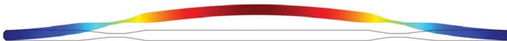
Figure 4. Optimized design for minimizing the cubic nonlinearity of a clamped-clamped beam and its linear vibration mode. The color in online version indicates the vibration amplitude.
