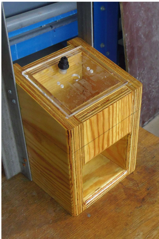
Fig. 5 The 1:50 scale model of one double-chamber section used in the DTU experiments. The tank wall was used as a symmetry plane, so only half of the section appears in the model. The water line is indicated by the black line
