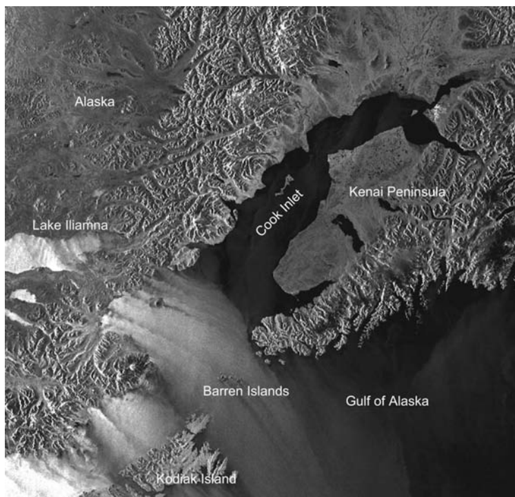
Figure 1. Radarsat-1 SAR NRCS image near Kodiak Island, Alaska. The bright or high cross-sectional areas represent high wind speeds. This image was acquired at 03:44 UTC on 31 October 2000 and was processed by the Alaska Satellite Facility. (Original SAR data courtesy of the Canadian Space Agency.)
