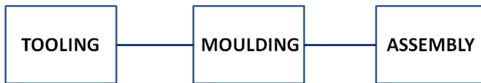
Figure 2 - Conventional Way of Manufacturing
