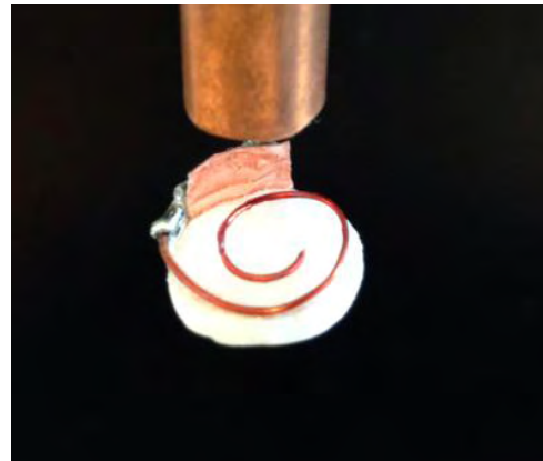
Fig. 1. The fabricated prototype of the spiral monopole antenna. The connected coaxial cable and balun are seen at the top.
