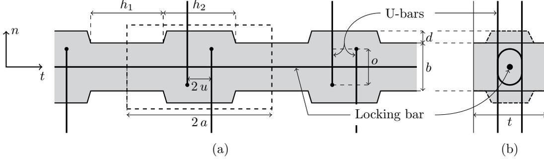
**Figure 2:** The basic design of a keyed joint reinforced with U-bars: a) elevation, b) cross section.
