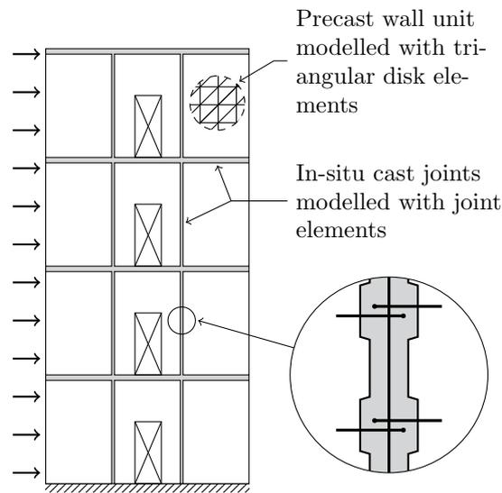
**Figure 1:** Four storey wall subjected to horizontal forces: The wall consists of 12 precast panels and joints. An example of a mesh (discretisation) for numerical analysis is seen for the top right panel.
