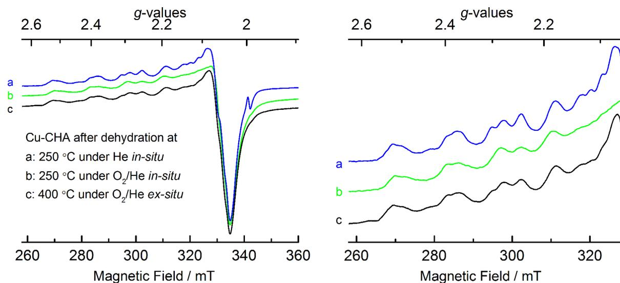
**Figure 3.** Comparison of EPR spectra of Cu-CHA after different dehydration methods. All spectra are collected at RT. (a) and (c) are collected under He atmosphere, and (b) is collected under an  $O_2/He$  atmosphere. The small peak at  $g = 2.0$  in spectrum (a) was identified as coming from the thermocouple which had entered the cavity of the EPR instrument slightly in this particular experiment. The signal is not from the sample. A zoom-in of the same spectra is shown on the right.
