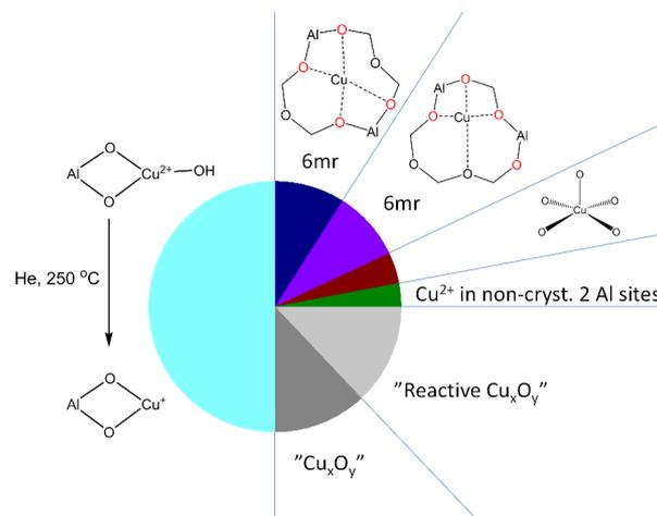
**Figure 7.** Speciation diagram of Cu-CHA after dehydration at  $250^\circ\text{C}$  showing the assignment of different species discernible by EPR using the in situ dehydration–rehydration method described in the text. The results for the EPR active species are largely the same as for the ex situ dehydration at  $400^\circ\text{C}$  in Table 1, except for the slightly lower total sum of EPR active species after the  $250^\circ\text{C}$  dehydrations.
