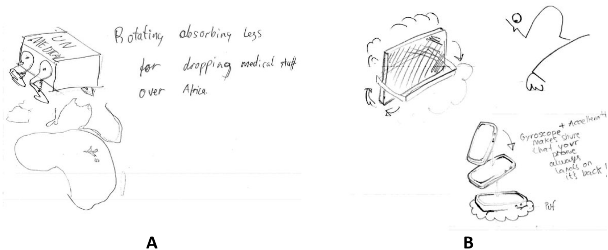
Figure 5. Two conceptual solutions for a collision protection mechanism inspired by the landing cat. (A) is inspired by the concrete biocard and (B) is inspired by the abstract biocard in Figure 4.
