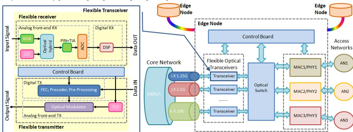
Fig. 2. Edge node architecture and detail of the flexible transceiver topology. VOA: variable optical attenuator, LO: local oscillator, ADC: analog-digital converter, TLS: tunable laser source, AN: access network.
