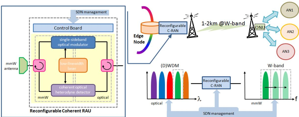
Fig. 3. Topology of a reconfigurable coherent RAU. C-RAN: coherent remote access unit, (D)WDM: (dense) wavelength division multiplexing.
