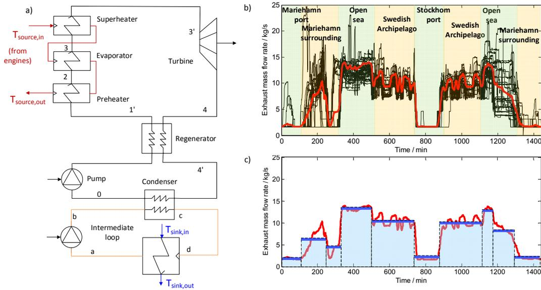
Fig. 1. a. Schema of the rORC model used in this work; b. Total estimated exhaust mass flow rate for different trips covering the same route as a function of time (black). The red line represents the average values from all the trips considered during the logged time. c. Approximation to the ship operation conditions in a return trip, where averaged values have been estimated to be used in the ORC model
