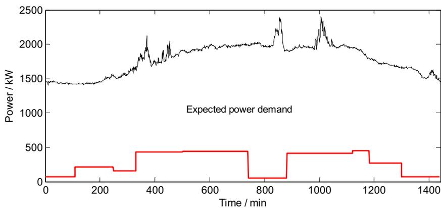
Fig. 2. Estimated net power production for the rORC (red line) and average logged values for the power demand on the ship (black line) during the average round trip.
