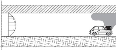
**Figure 8 – Schematic of tunnel without vehicular blockage.**
