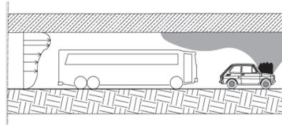
**Figure 9 – Schematic of tunnel with vehicular blockage.**
