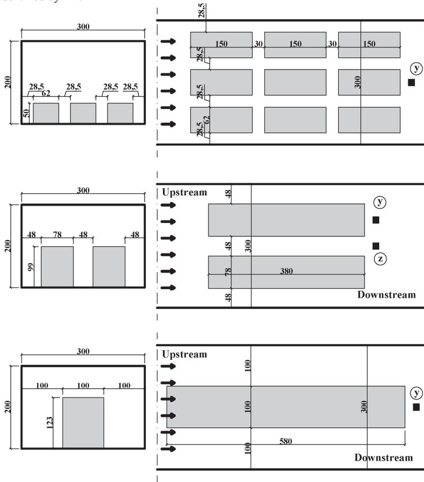
Figure 4 – Vehicular blockage models, A, B and C and fire source locations for scenarios set 1.
