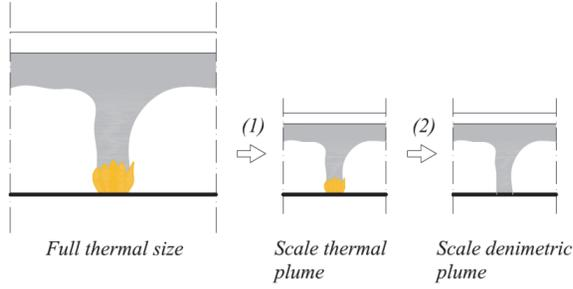
**Figure 1 – Principle of the two step-scaling, [28].**
