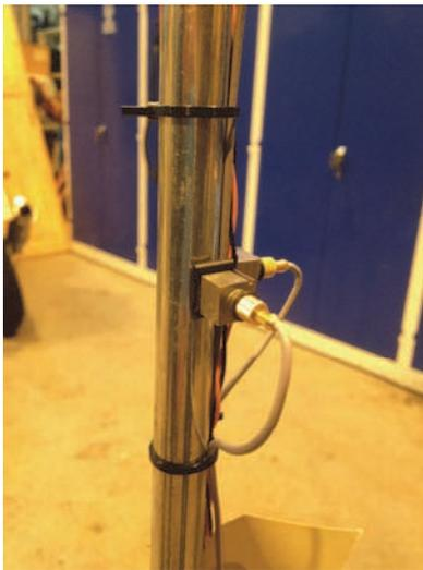
Fig. 6: Accelerometer mounting at the mid tower.
