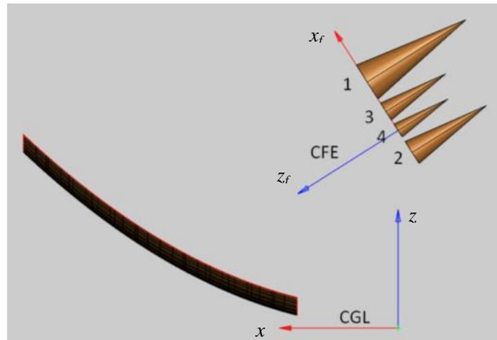
Figure 3: Definition of the global coordinate system (CGL) and feed cluster coordinate system (CFE) with origin in center of horn 4.
