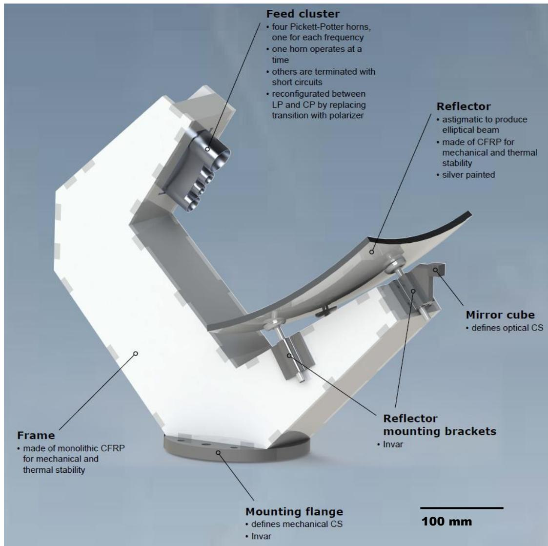
Figure 2: The DTU-ESA Millimeter-Wave Validation Standard Antenna (mm-VAST).
