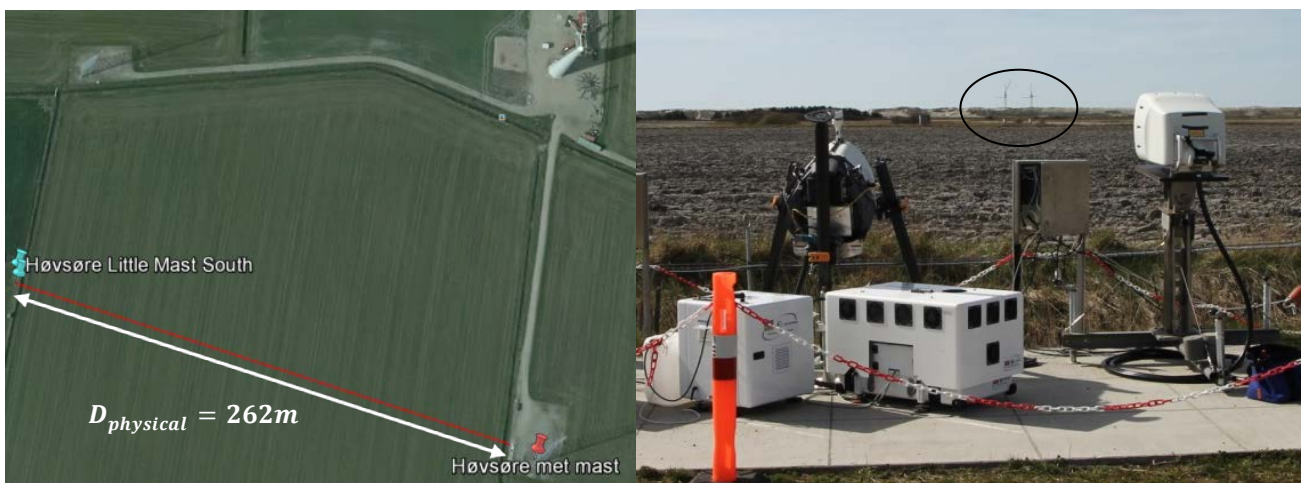
Figure 5. Calibration measurement setup of ZDM (ZephIR) and the 5-beam Demonstrator (Avent) at DTU Wind Energy test site, Høvsøre (DK)
