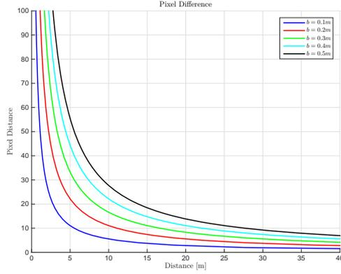
Fig. 10. Theoretical Pixel values as function of distance
