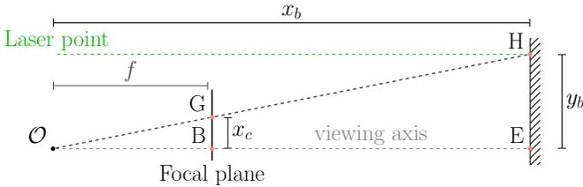
Fig. 4. Top view of the laser sensor triangulation
