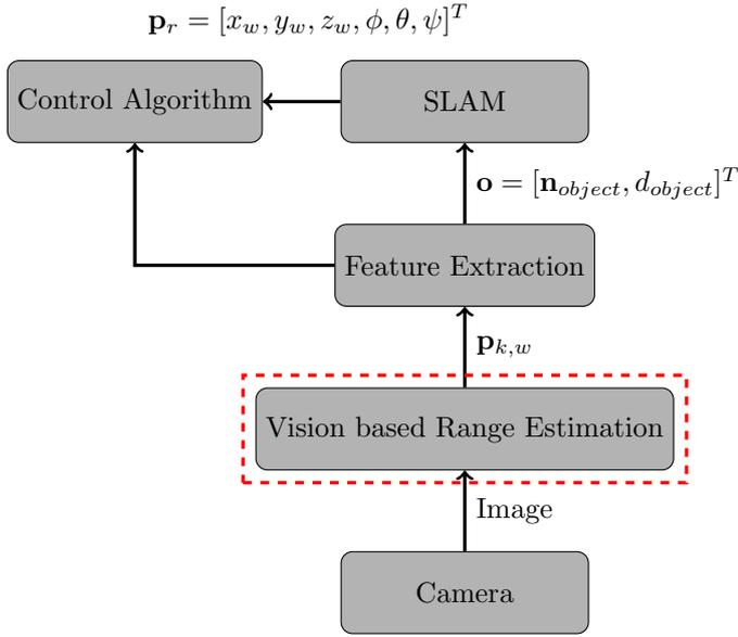
Fig. 1. Overview of the robotic control architecture
